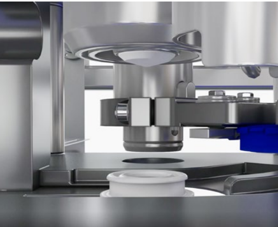
Fill head unit is capable of maintaining sterility throughout uncapping, filling, and recapping.
