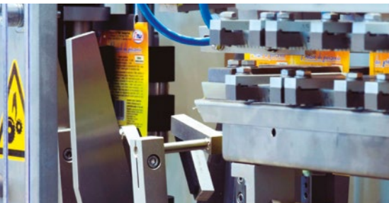
This model in duplex version, includes two independent vertical sealing groups.
