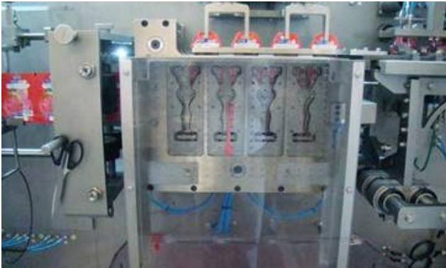
Cutting die allows for pouches with total shape.
